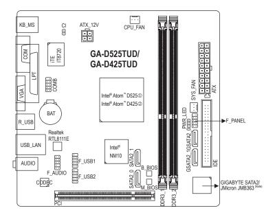
(Note) When installing Windows XP onto the hard drive connected to the JMicron JMB363 controller, be sure to connect the optical drive to a SATA port controlled by the Intel chipset.
