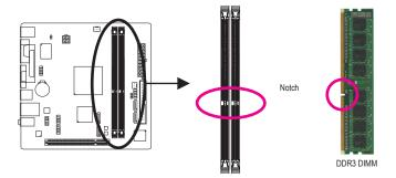
A DDR3 memory module has a notch, so it can only fit in one direction. Follow the steps below to correctly install your memory modules in the memory sockets.
