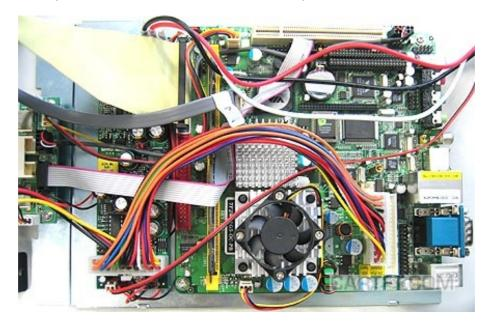
The ATX-cable should be laid like shown in the picture:
