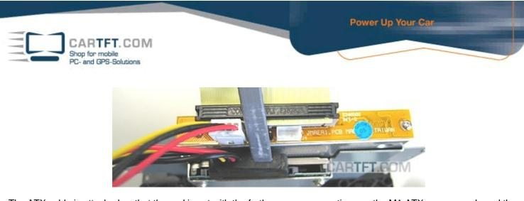
The ATX cable is attached so that the end is put with the further power connections on the M1-ATX power supply and the other one end on the motherboard. The ATX cable or all other cables, too, have to be laid flat, compact and space-saving, so that the floor metal can be put into the VoomPC-2 enclosure without problems. This is what it should look like:
