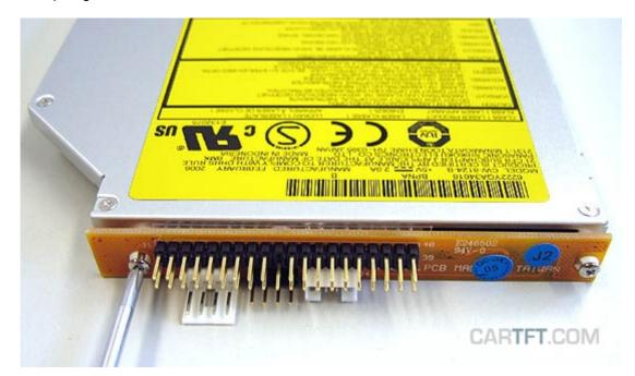
Then the CD/DVD drive gets installed at the drive mounting unit, which gets screwed at the side with 2 small screws:
