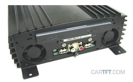
At the rear the power connector cable gets led out and put it into the rear faceplate.
