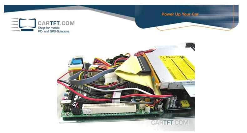
The floor metal gets pushed with the drive mounting unit into the enclosure carefully, so that no cable gets stuck or gets damaged.
