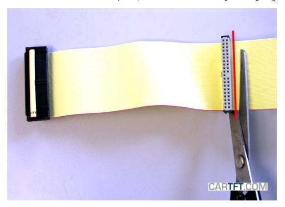
Connect the 2,5" to 3,5" adapter to the HDD, as well as also the included IDE-cable shown in the first following picture. After that you buckle the IDE cable shown like in the second picture:
