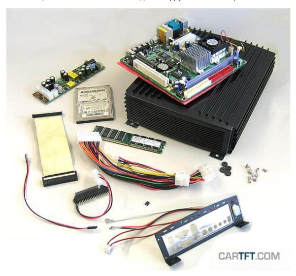
The floor metal is pulled out of the case and the motherboard is attached on it. You screw in a bit all 4 screws, but before screwing them tight you have to push the motherboard into the shown direction shown in the picture for winning more space for the HDD and the power supply later.
