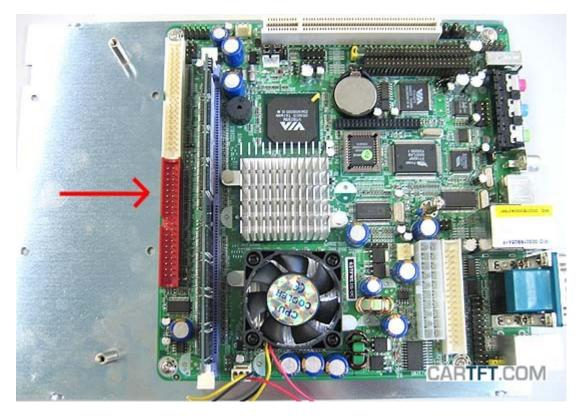
The IDE-cable is cut like shown in the picture, the rest of the cable on the right side is garbage:
