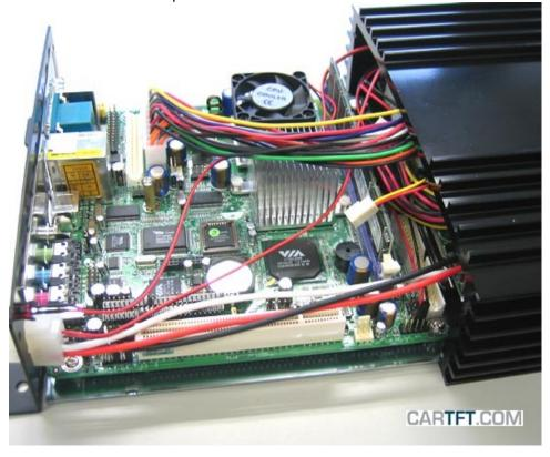
The case ventilator (Sysfan) is finally put on its place.
