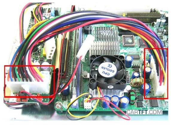
You attach the HDD electric cable to the ATX current plug, already in the direction of the HDD electric cable shows to it. The other two ATX electric cables (Floppy and CD/DVD disk drive) are bent, packed and kept flat as well as possible:
