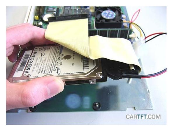
You screw in tight the hard disk and connect the IDE cable with the next IDE port. The hard disk electric cable from the 2.5 "on 3.5" adapter is put inside around the small post:
