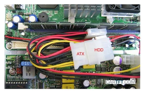
The following picture shall clarify that the ATX cable or also all other cables must be kept flat so that one gets the floor metal into the VOOM case afterward:
