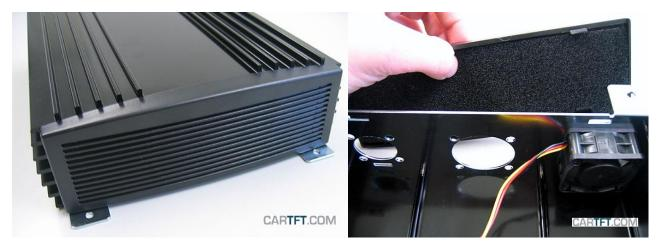
Now the case ventilator is placed from the outside...into the middle:
